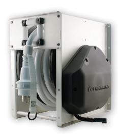
These self contained 'ready to fit' systems feature an innovative clutch mechanism that allows the storage reel to 'free wheel' making it easy and quick to use - simply pull out whatever length of shore power cable is required, and when its time to retract the cable, press and hold the control switch (supplied) to engage the powerful DC motor (12v or 24v) that will effortlessly retract the cable and re-store it on the reel.
